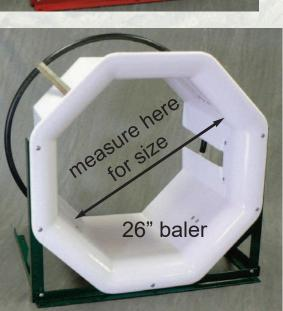
and sizes), or by measuring diagonally across the inside from corner to corner, (see photo of 23" baler, left).
