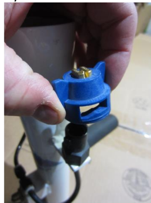
Turn Nozzle body ¼ turn counterclockwise to remove spray tip body
