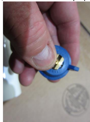
Push Spray Tip down and remove from body
