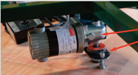
direct drive motor and slip clutch shown
