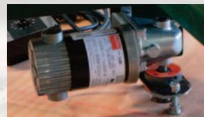
Turn Table Motor and Clutch Assembly, includes plate, slip clutch and wire terminals:
