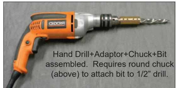
Hand Drill+Adaptor+Chuck+Bit assembled. Requires round chuck (above) to attach bit to 1/2" drill.
