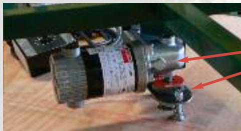
Inverted view of turn table drive
